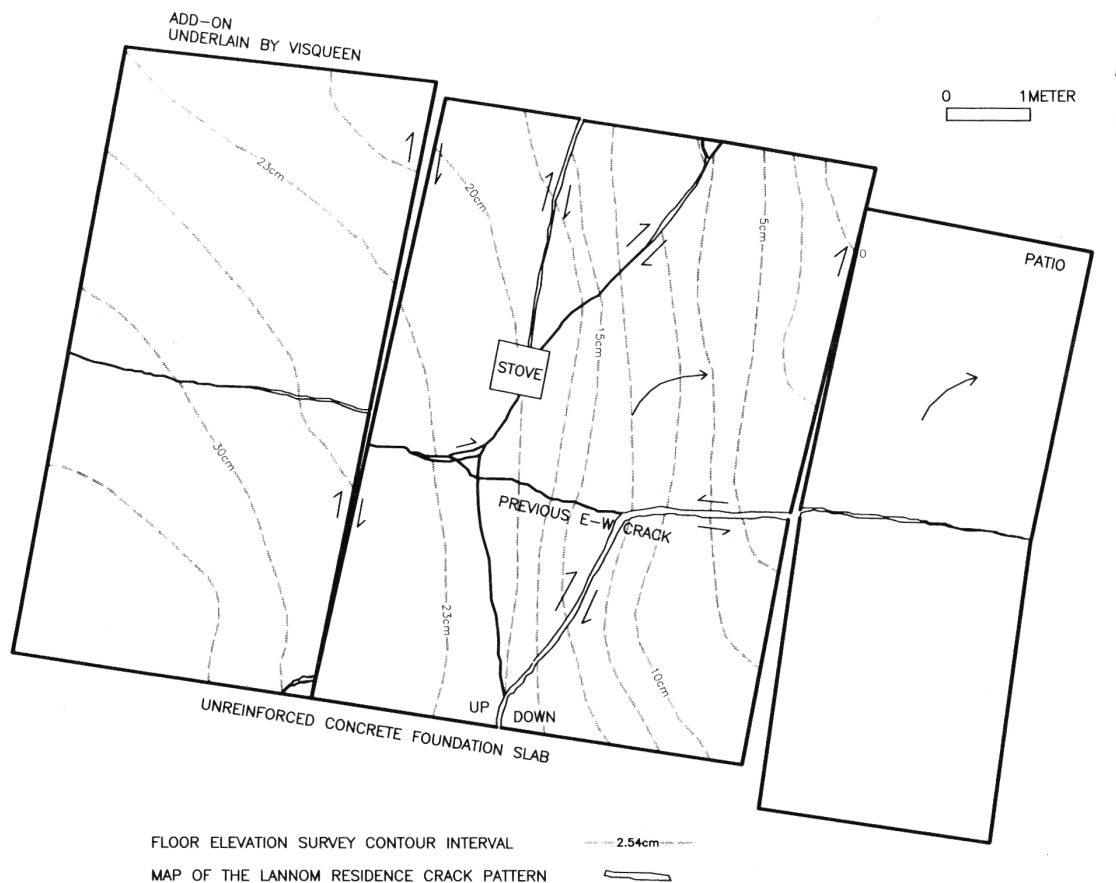
Figure 6 Deformation of foundation slab of Lannom residence. Left unreinforced concrete foundation slab is underlain with plastic (Visqueen) and right foundation slab is not underlain with plastic. Primary fault scarp is to the left of this building (after Murbach et al. 1999).
